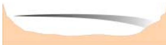
Diagram 16: Significant vertical density differentiation as the result of temperature gradients caused by sunlight
